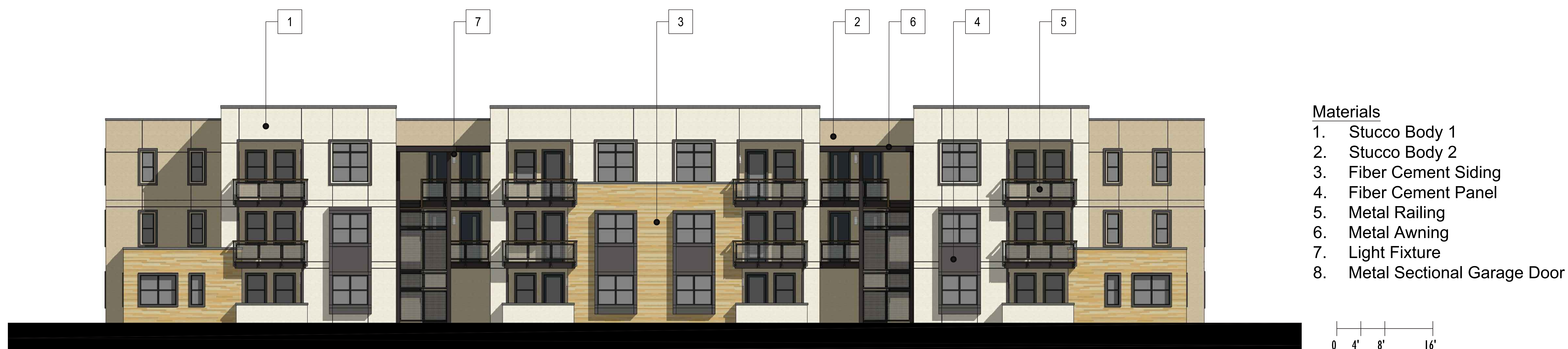
Figure 3, Conceptual Residential Front Elevation
