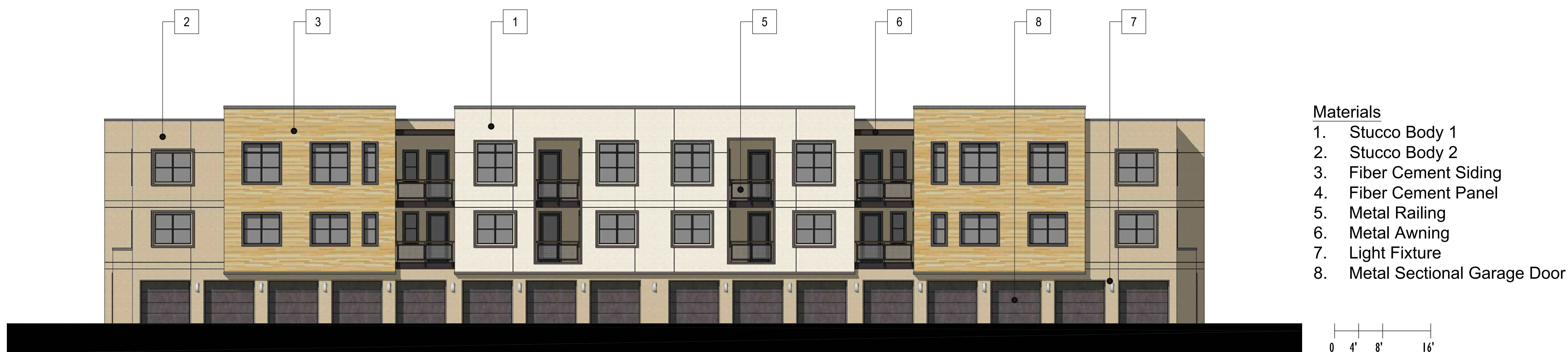
Figure 6, Conceptual Residential Rear Elevation
