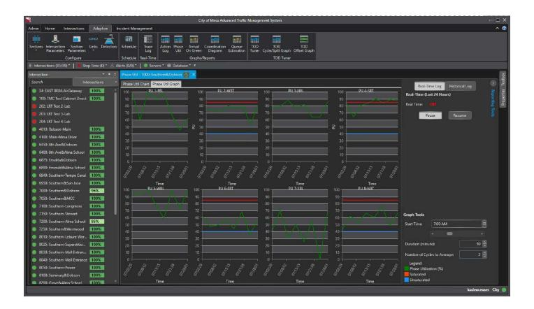
The cycle tuning algorithm used in Kadence extends from a "critical intersection" algorithm. The phases that are designated to be checked in the cycle tuning algorithm are determined by the user. When the average phase utilization on these critical phases is above the user-defined threshold (say, 80% phase utilization) to increase the cycle, a given (the user-defined step size) number of
