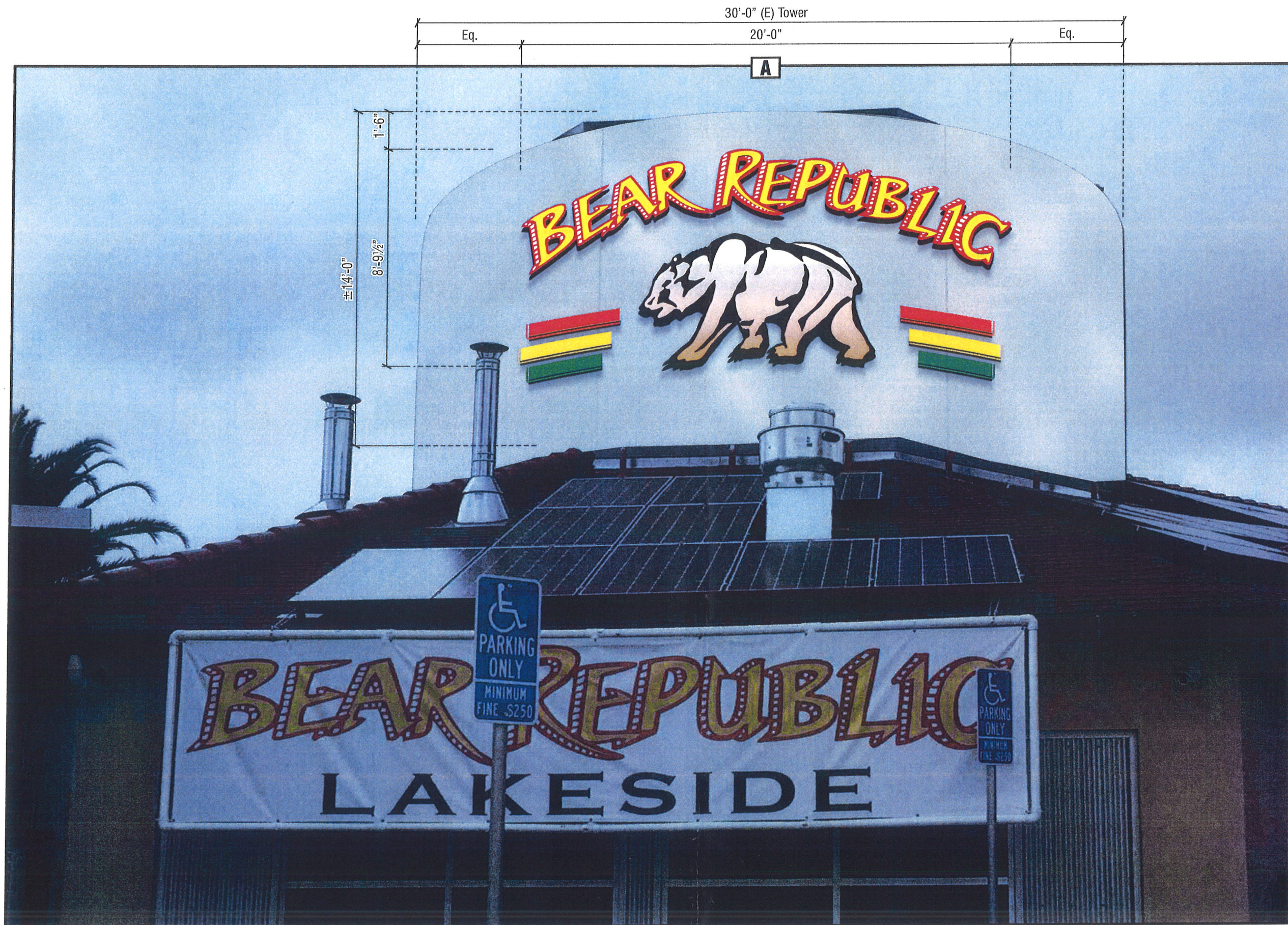
1 STOREFRONT ELEVATION @ TOWER - PROPOSED CUSTOM FABRICATED CURVED DUAL-ILLUMINATED CHANNEL LETTER & PLAQUE SIGN Scale: Approx. 1/4" = 1'-0"
